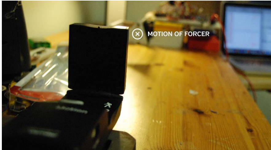
Fig 10. The motion detector (foreground, left) pointed at the back of the forcer (background, white triangle). The forcer recesses from the sensor (goes into the page).
